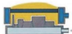
4 加砂震实 sand compaction
