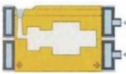
7 待浇注的铸型 Combine the two flasks
